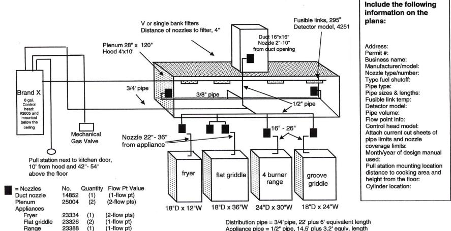
NOTE: Used the 1/2004 issue of Brand X design manual. Total nozzle flow pt. count = 12, Total flow pt. count allowed = 14
